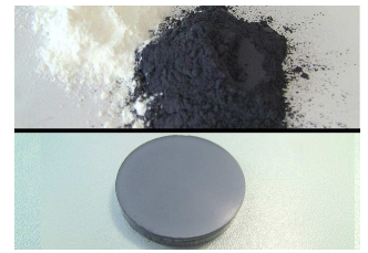
FeSiMg-Granulate 12 g plus 2 g licowax Particle size 0.10 mm Pressing tool 40 mm Aluminum cups 60 s 15/25/35 tons
