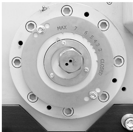
Scale for continuous gap width setting
