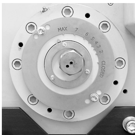
Scale for continuous gap width setting
