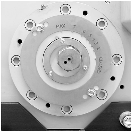
Scale for continuous gap width setting
