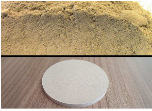
Wood 4g Particle size 0.25 mm Pressing tool 32 mm 20 s each at 10/20/30 tons
