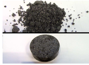
Slag 40 g Particle size 0.25 mm Pressing tool 40 mm 20 s 20 tons
