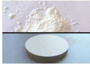
Cellulose 7 g Particle size 0.15 mm Pressing tool 40 mm Aluminum cups 40 mm 30 s each at 10/20/30 tons
